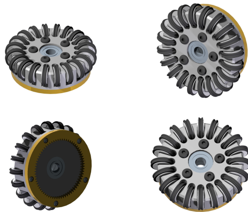
Fig. 3. Different views for the computational model of the new wheels of the STOx's 3 rd generation. Its diameter is larger than that of previous generations and it contains 5 more rollers
