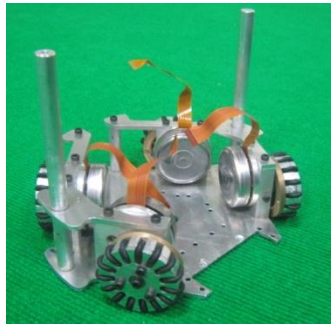
Fig. 2. Robot's chassis with wheels and motors
